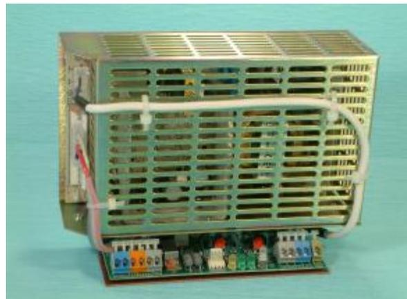
**Fuses: F1 (connected in L+), F2 (connected in B+), value 6.3A/250V**
