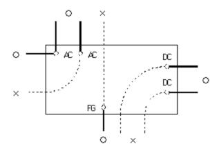
Avoid laying out the AC input line pattern directly beneath the power supply as it will increase the line conducted noise. Make sure to leave ample distance between the line pattern underneath the unit because the output noise may increase. Seprate the pattern lay out form the unit.
