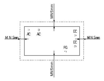
When installing the components or laying out the pattern around the unit, maintain a distance of 5mm or more. If this distance can not be kept, insert an insulation sheet between them.
