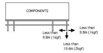
When too much stress is applied on the input/output/FG pins of the unit, the internal connection may be weakened. Avoid applying stress of more than 9.8N (1kg) on the pins horizontally and more than 19.6N (2kg) vertically. When additional stress is expected to be put on the input/output pins because of vibration or impact, fix the unit to PCB using silicone rubber or another fixing method to hold stationary. This will reduce the stress onto the input/output pins.
