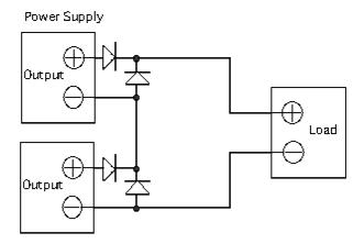
These power supplies can be used in parallel operation as shown below.
