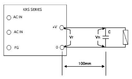
Vr: Testing point of output voltage, output regulation.
