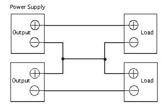
These power supplies can be used in parallel operation as shown below.
