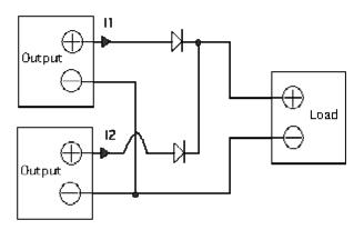
In order for the two power supplies to share the load accurately, it is important that both output voltage remain identical under all load and line conditions. This is necessary to prevent any unbalanced current sharing.
