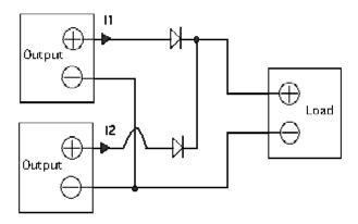
In order for the two power supplies to share the load accurately, it is important that both output voltage remain identical under all load and line conceives. This is necessary to prevent any unbalanced current sharing.
